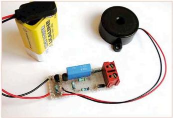
Under normal circumstances, the voltage across R3 is high enough to keep T1 in conductance. The gate of T2 receives a too small voltage to keep this MOSFET conducting so no current from the battery
