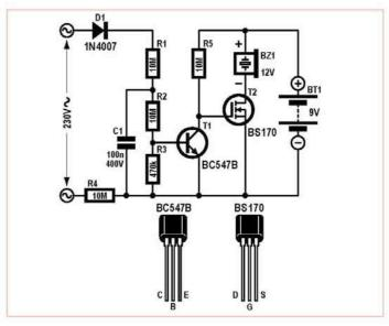
of the prototyping board). Here we should repeat that it is critical to use resistors which can handle voltages up to 350 V for R1 through R4, and a 400-V rated capacitor for position C1.
